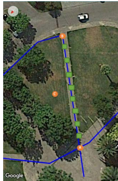
Figure 6. Example of filling intermediary points to determine the closest segment to a given point
