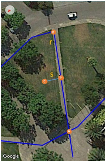
Figure 5. Example of finding the point in a segment that is closest to a GPS location
